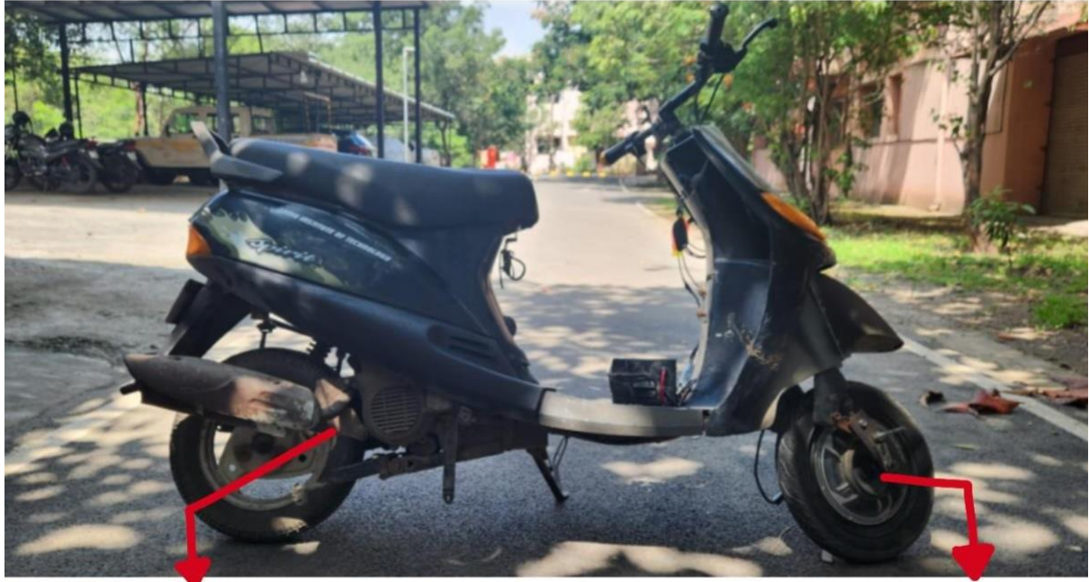
Electric Hub motor to drive front wheel.
