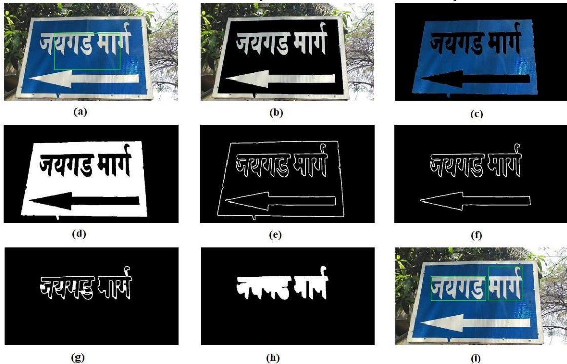
Figure 3. Combined approach with arrow removal (a) Selected center area (b) Objects in cluster one (c) Objects in cluster two (d) Randomly selected cluster (e) Edge detection and gradient mask (f) Region-based filtering (g) Arrow removal (h) Region-filling and CC analysis (i) Detected text.
