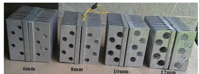
Fig. 2. Photo image of different types of perforation size with zigzag perforation configurations [41].
