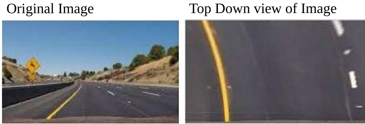
Fig. 2 Inverse perspective transformation
